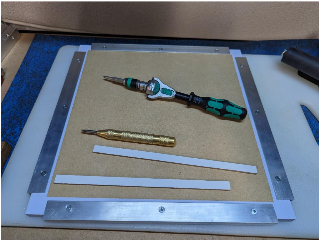
The base tiles should sit nicely side by side and the join can be covered with the vinyl topped Aluminium Channel (U shape profile) sections.
